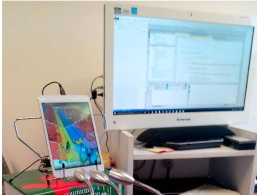
Fig. 9. GeoLiFi Kit Android Tablet 4.2.4 and three Li-Fi lamps.
